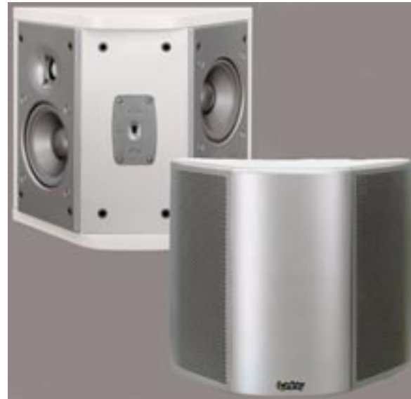
Figure 6. An Infinity Beta ES250 wall-mounted surround loudspeaker, with a switch to select the directional mode: monopole, bipole or dipole. The customer can use the mode appropriate to the application, the room, or personal preference. The two active faces can also be driven independently, for special situations.
